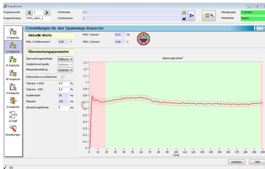
Fig. 2-8 X-Pegasus representation with open U-Inspector settings
