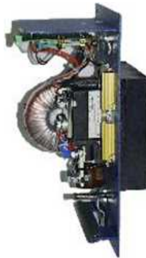
Fig. 11-3 LE100-Thyristor power stage
