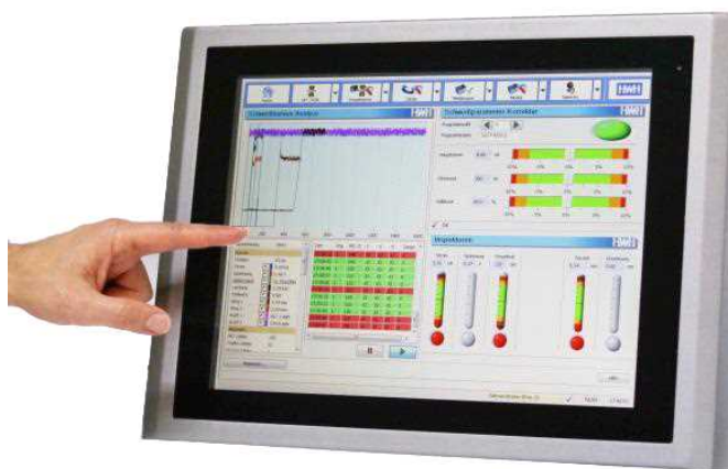
Fig. 3-1 Xcomand2.1 - the color touch display
