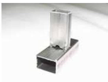
Fig. 12-6 Welding hollow sections
